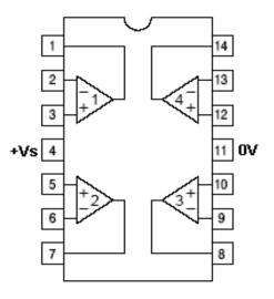
Figure 3 Pin Configuration of LM 324 amplifiers IC
