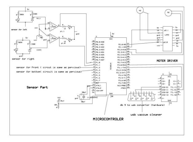
Figure 8 Circuit diagram of microcontroller based Robo Cleaner
