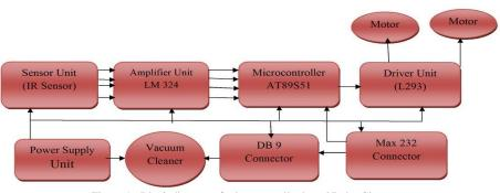
Figure 1 Block diagram of microcontroller based Robo Cleaner www.ijarcce.com
