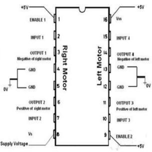
Figure 6 Interfacing driver IC and stepper motor[10]
