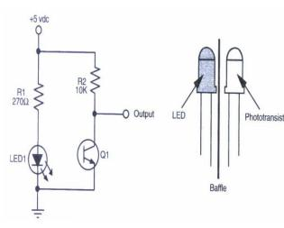
Figure 4 Basic design of the infrared proximity sensor [7]
